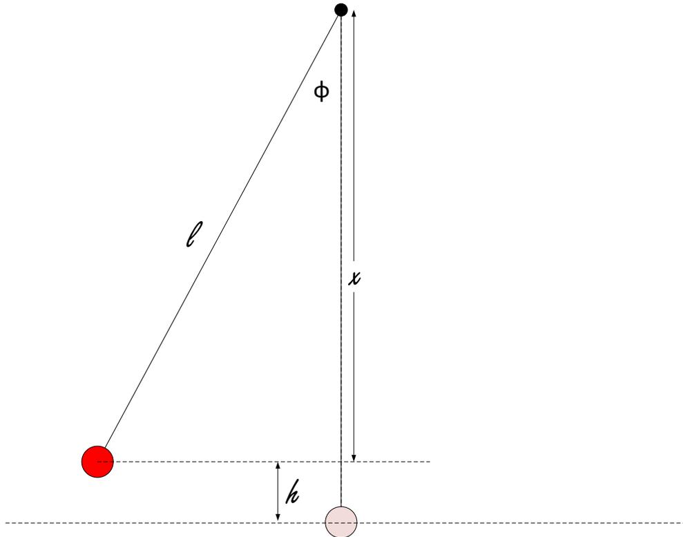
The pink weight indicates the position of the weight at its lowest point. Note we have a right-angle triangle with  $l$  being the hypotenuse and  $x$  being the adjacent to angle  $\phi$ . Therefore, the length of  $x$  is:
