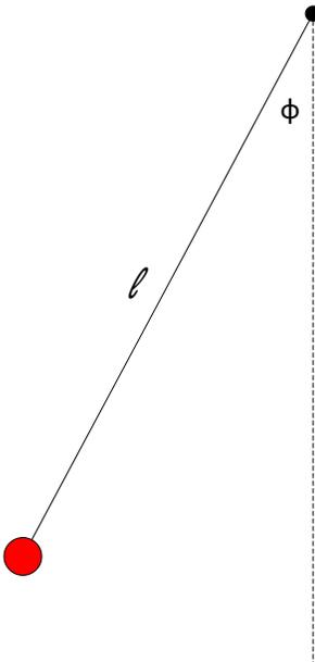
At this position of motion, the red weight is not moving resulting in 0 kinetic energy and the potential energy is all that exists at this point. To derive that energy, we apply the formula:
